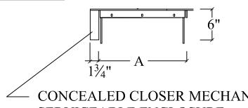
CONCEALED CLOSER MECHANISM INSIDER SERVICEABLE ENCLOSURE
