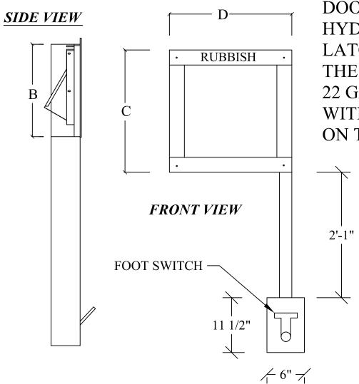
DOORS COMPLETE WITH SELF CLOSING HYDRAULIC CYLINDERS, SELF LATCHING TRIGGER ASSEMBLY THE DOOR FRAME IS COVERED WITH 22 GA. STAINLESS STEEL NO.4 FINISH WITH EMBOSS LETTERING "RUBBISH" ON TOP OF TRIM PIECE
